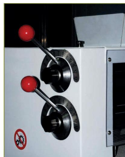
Detail of adjustment levers for laminating thickness
