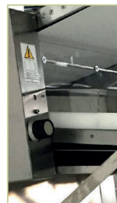
Detail of control knob for thickness adjustment
