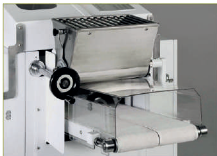
Detail of a 2-way delivery on the front and stainless flour duster
