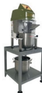
Supporting frame with shelf for tools - adjustable feet
